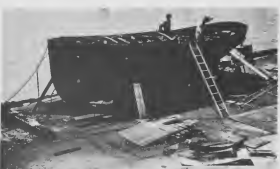
HAMMERS AND torches are being used on a stripped-down workday of the harbor, known affectionately as Mooring Launch Number 2. She's getting a new gunwale and deck housing, and other needed repairs next to other projects at the drydock.
